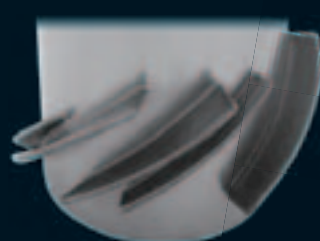
Helical deposition (Near net shape) - Steel substrate parent material - Inconel 718 deposition material
